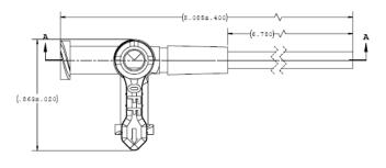
**Reason:** Nordson Medical part number FCA026-001 stopcock tubing assembly can crack at the tubing bond location. These cracks are determined to be due to high molded-in stresses within the polycarbonate housing, eventually relieved when a solvent is used to bond the tubing. Root cause and problem solving analyses has proven that annealing the stopcock housings is the solution.
