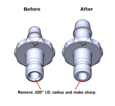
**Reason:** The BPM male bayonet connector is being updated to conform to the upcoming ISO80369-5 standard. To learn more about ISO80369 (an initiative by a joint working group established by the ISO and International Electrotechnical Commission) standards and its objective of preventing misconnections in health care settings, please visit http://www.nordsonmedical.com/products/iso\_80369.aspx
