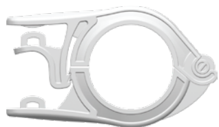
CPAX150 (-U71, -U75, -U706) Tri-Clover Easy-Open Clamp for Maxi Flange, 1" (25.4 mm) to 1.5" (38.1 mm), Glass-Reinforced White, Blue, or Orange Nylon
