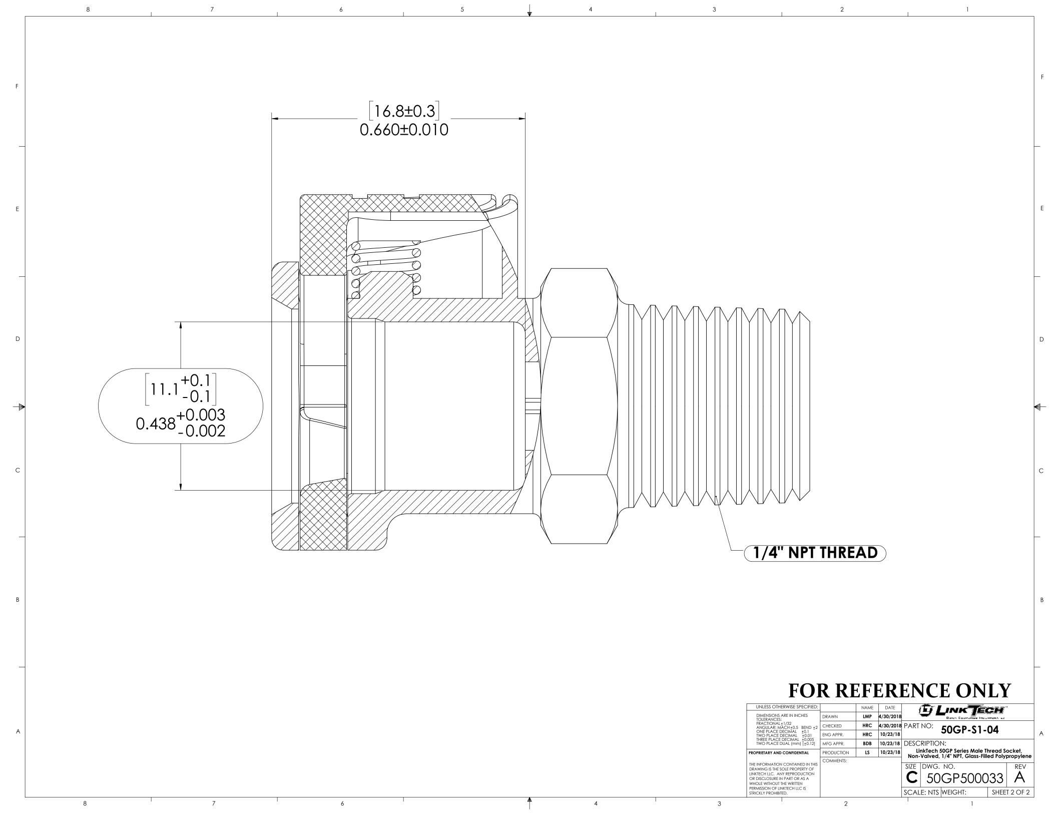
REVISIONS DESCRIPTION APPROVED UPDATE DWG TO CURRENT FORMAT & STANDARDS 10/23/2018 LATCH (ACETAL) -SOCKET (GLASS-FILLED POLYPROPYLENE) [35.6] 1.40 [23.5] 0.93 1/4" NPT (PIPE THREAD) LATCH SPRING, **INTERNAL** (STAINLESS STEEL) FOR REFERENCE ONLY UNLESS OTHERWISE SPECIFIED: LINK TECH DIMENSIONS ARE IN INCHES
