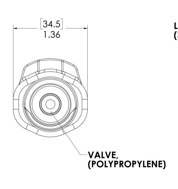
70.6±0.8 LATCH SPRING, (STAINLESS STEEL) 2.78±0.03 [10.7] Ø 0.42 [36.6] 1.44 3/8" TUBE ID VALVE O-RING, **INTERNAL** (EPDM) VALVE SPRING, INTERNAL (STAINLESS STEEL)
