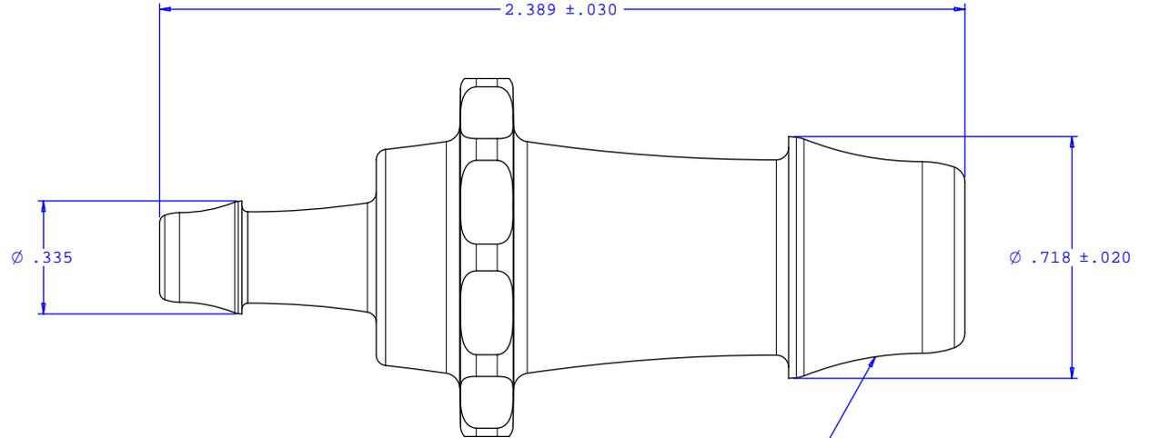
2X INSTRUMENT QUALITY PART. NO PARTING LINE PERMITTED ON THIS CONICAL SURFACE
